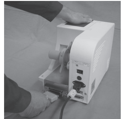
Align the interface board with the guide of the interface slot opening.
